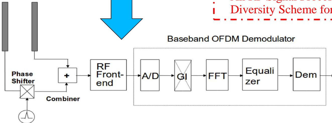
An RF Signal Processing Based Diversity Scheme for OFDM Systems
